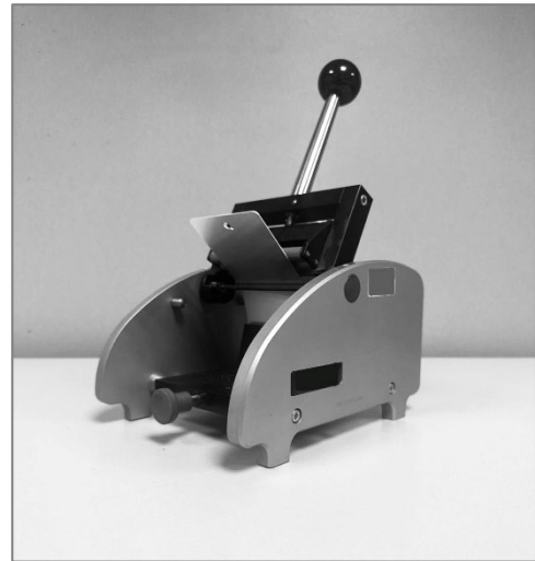
Figure 4 – Apparatus for testing the resistance to cracking on bending
