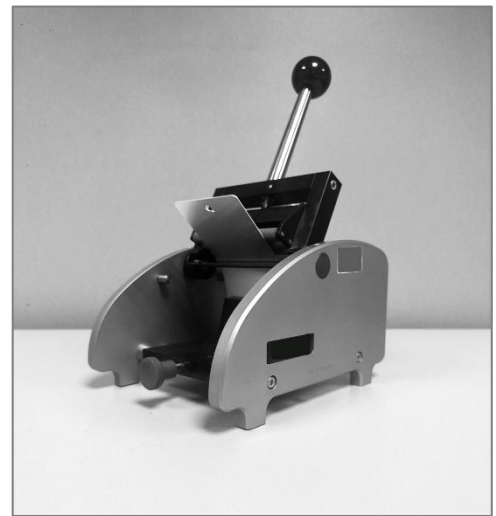
Figure 5 - Apparatus for testing the resistance to cracking on bending
