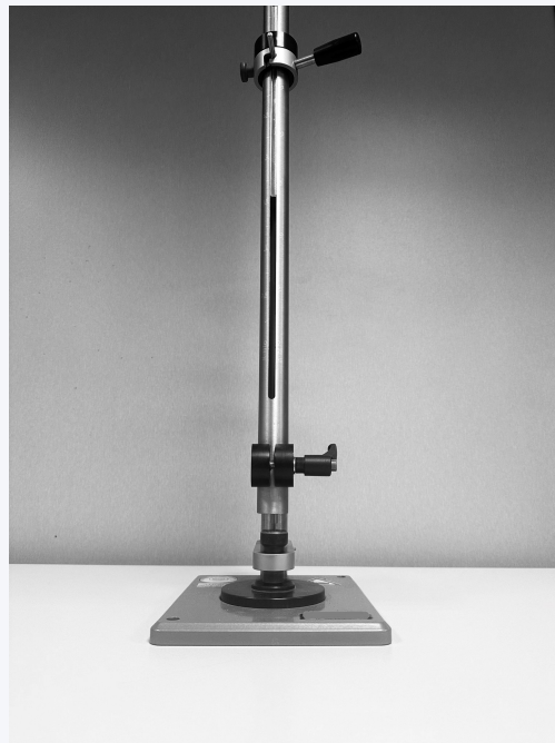
Figure 6 - Apparatus for impact test
