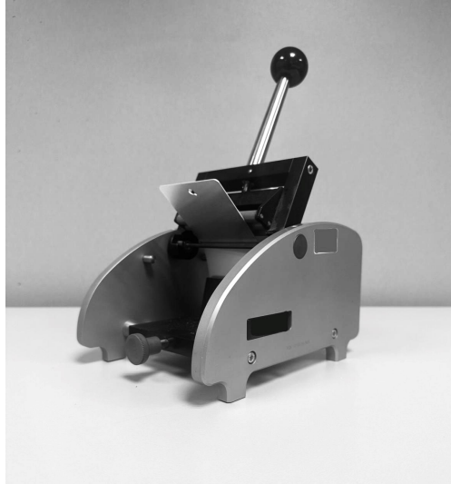
Figure 8 - Apparatus for bend test
