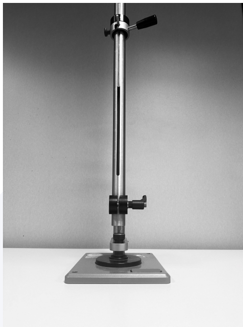
Figure 11 - Apparatus for impact test
